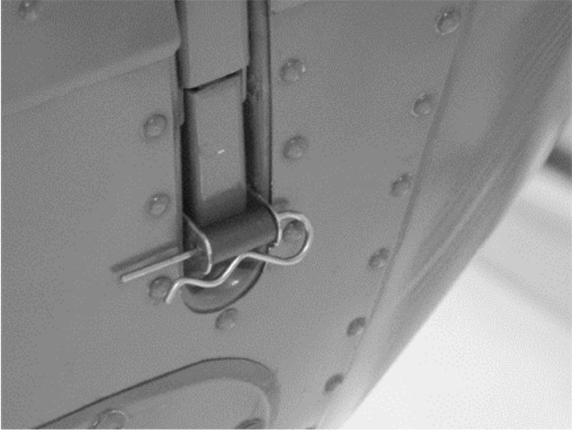
The spacer also helps keep the lower arm of the latch snapped on its spring catch. The pin firmly pinches the spacer so the pin does not slide fore and aft, preventing wear on the bottom left and right edges of the retainer – two more benefits. With thanks to Fred and Steve!
