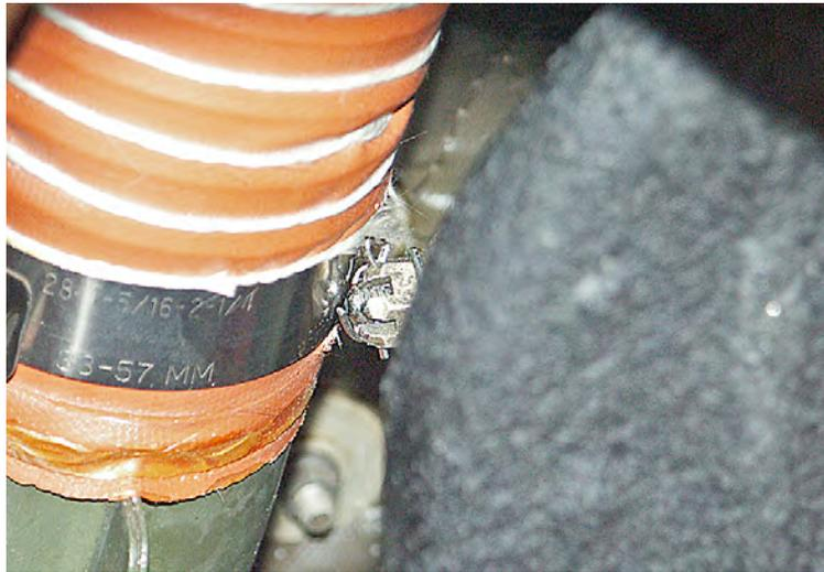
Reversing the AN3H37 bolt so the *head* is adjacent to the duct fitting, as shown in Fig. 159 of the same parts manual, provides the necessary clearance for full pedal travel. Conflicting info in a Birddog manual? Who'd believe that?
